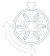
Figure 12: Bouton set du thermostat
